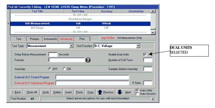
When the test is run using ProCal, the voltage measured will be displayed as a current (amps) reading.
